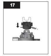
• Connect the sleeve bolt to the top of the sleeve assembly.
