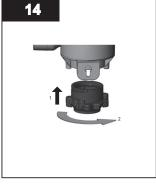
Connect the sleeve bolt at the bottom of the sleeve assembly.
