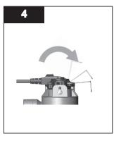
• Pinch wire form to release the safety cap.
