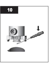
• Pry sleeve upwards using sleeve removal tool until it comes loose.
