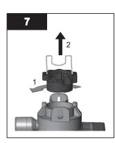
• Remove the sleeve bolt from top of the sleeve assembly.
