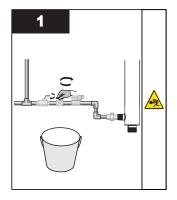
• Shut off the water line to chamber and release system pressure before servicing.
